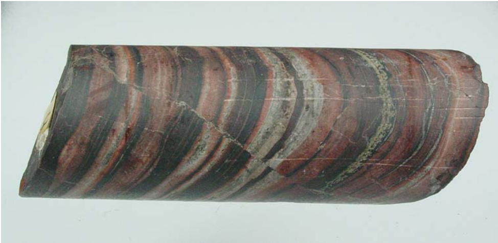
Sphalerite (light grey) with abundant inclusions of chalcopyrite
